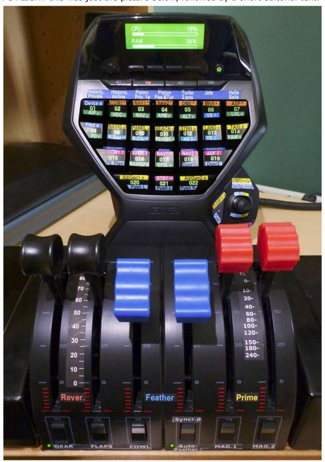
"Club Member Claudio Di Veroli managed to install the Logitech G13 onto the back of the Saitek dual throttles. Note how the throttle scales is graduated from 0 to 100%, the Mixture is graduated according to FL (in FS9, this optimum mixture at a given altitude is the same for all the piston engine aircraft). On the G13 he has loaded 3 routines:
